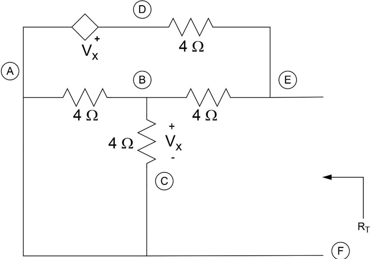
Solution: (Self Assessment) The input resistance  $R_T = 3$  ohms.
