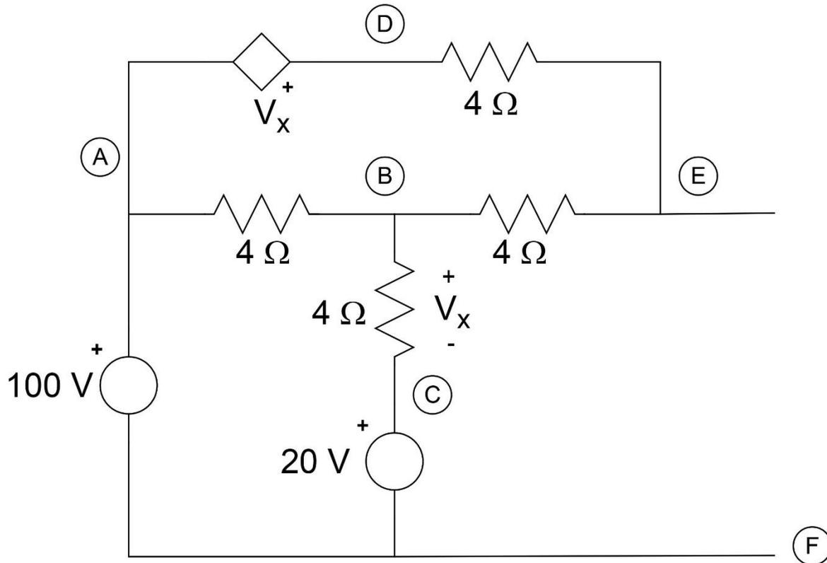
Solution: (Self Assessment) The open-circuit voltage  $V_{EF} = 120$  V.
